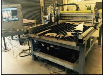
Building a precision cutting tool from salvaged parts enables the Village Creek Water Reclamation Facility (Fort Worth, Texas) to make the custom pieces it needs for repairs. Credit: Village Creek Water Reclamation Facility
